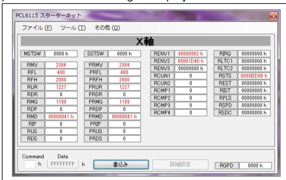
Output pulse specification (PMD2 to 0) of the environment setting 1 register (RENV1): 0 x 03.
