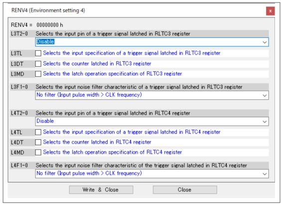
Select the desired setting state from the pull-down menu, check menu, and click the "Write & Close" button. Write to RENV4 register and close "RENV4 (Environment setting 4)" menu screen.
