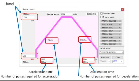
Pulses are calculated by integers, so a motion profile may not be realized as specified values. Also, if you set an impossible value, an error will be displayed.
