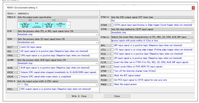
Select the desired setting state from the pull-down menu and check menu and click the "Write & Close" button. Write to RENV1 register and close "RENV1 (Environment setting 1)" menu screen.
