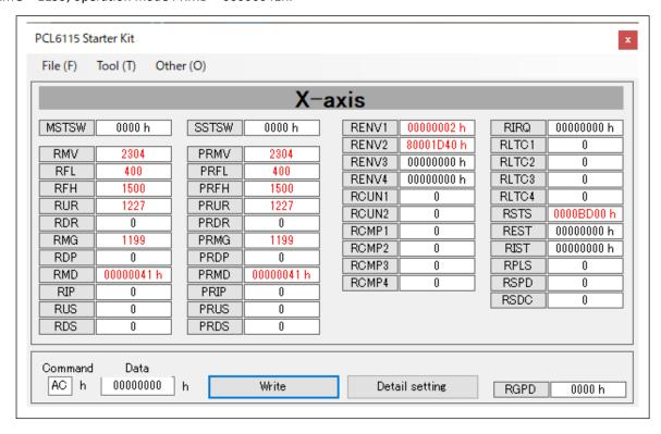
To set a value to PRMG, the setting menu is displayed by clicking the "Detail setting" button. Set a magnification rate to 1 and click the "Write & Close" button.
