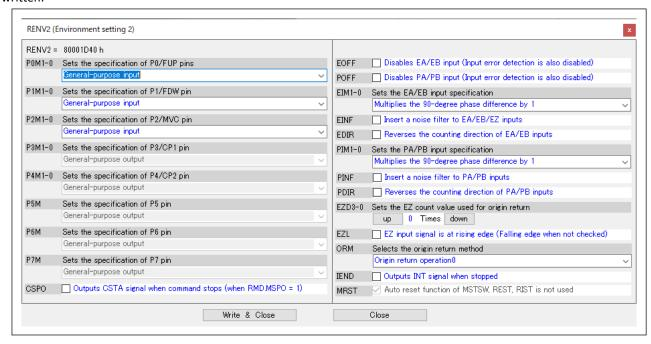
Select the desired setting state from the pull-down menu and check menu and click the "Write & Close" button. Write to RENV2 register and close "RENV2 (Environment setting 2)" menu screen.
