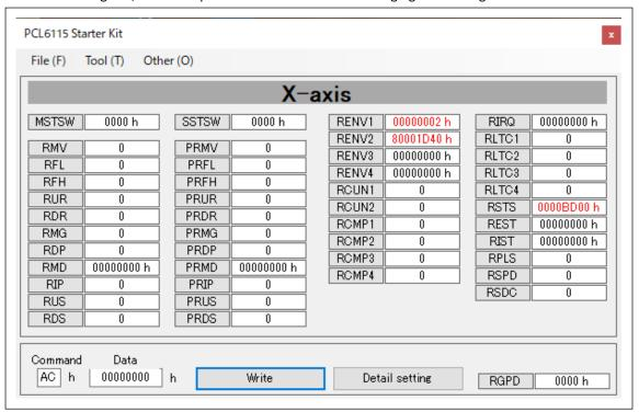
For PRMV setting value, write a value that an output shaft of a stepping motor PFCU30-24V4GM (1/12) rotates once.
