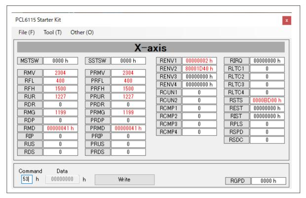
Write a start command 53h in the column "Command" and click the "Write button.
