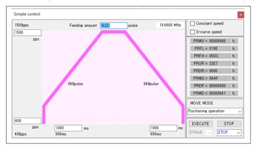
Close the "Simple control (M)" menu screen by clicking the "Close" button or close mark at the upper right corner.
