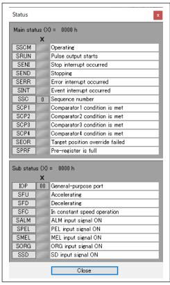
Bit items that are set to "1" in registers are displayed in blue. Close the "Status" menu screen by pressing the "Close" button.
