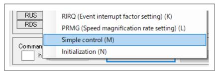
Click the "Simple control (M)" menu to display Axis in the following screen. You can set an operation pattern to perform a simple motion control.
