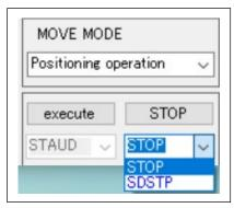
After setting the operation pattern, when you click the "EXECUTE" button, the value of each register is written to PCL6115, and the set operation is performed once. At this time, "FH high speed start" (STAUD: 53h) is written to PCL6115 as a start command for linear control and S-curve control, and "FL constant speed start" (STAFL: 50h) is written to PCL6115 for constant speed control.
