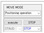
"MOVE MODE " can be selected from 5 operations "Positioning operation", "+ direction continuous operation", "- direction continuous operation", "+ direction origin return operation", and "- direction origin return operation".
