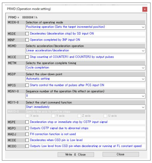
Select a desired setting state from the pull-down menu, check menu, and click the "Write & Close" button. Write to PRMD (or RMD) register and close "PRMD (Operation mode)" menu screen.
